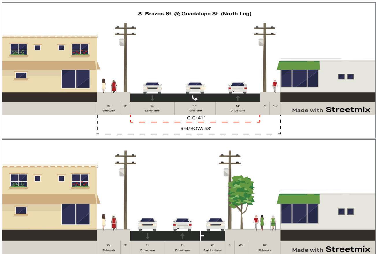
Figure 13: Existing and Proposed Cross-Section - North of Guadalupe Alternative 1
