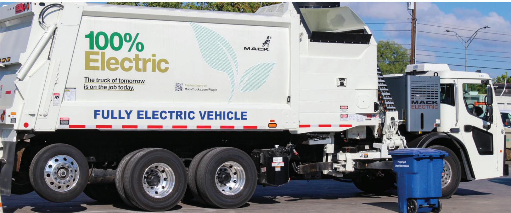
The Department scheduled demos of two different electric garbage trucks in 2022. The first was a Mack LRE chassis with a Heil body. It started off at a VIA Transit Center where the required 480-volt plug was located. Beginning at an 8% charge, the truck took 14 hours to fully charge. The truck picked up roughly 240 carts, made two trips to the landfill and dumped about two tons of material.
