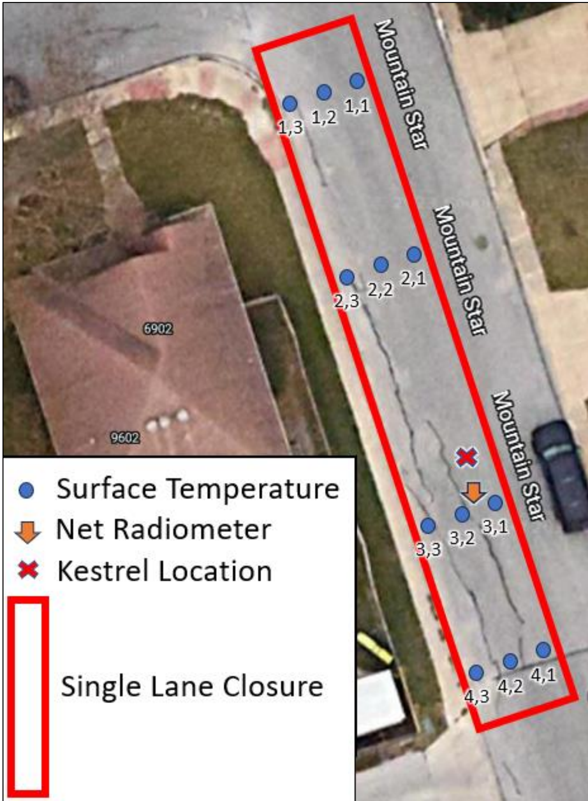
Figure B5. Fieldwork data collection schematic for the Mountain Star cool pavement site showing the surface temperature grid and Kestrel location during Phase I and the net radiometer location during Phase II (Imagery Source: Google Maps).
