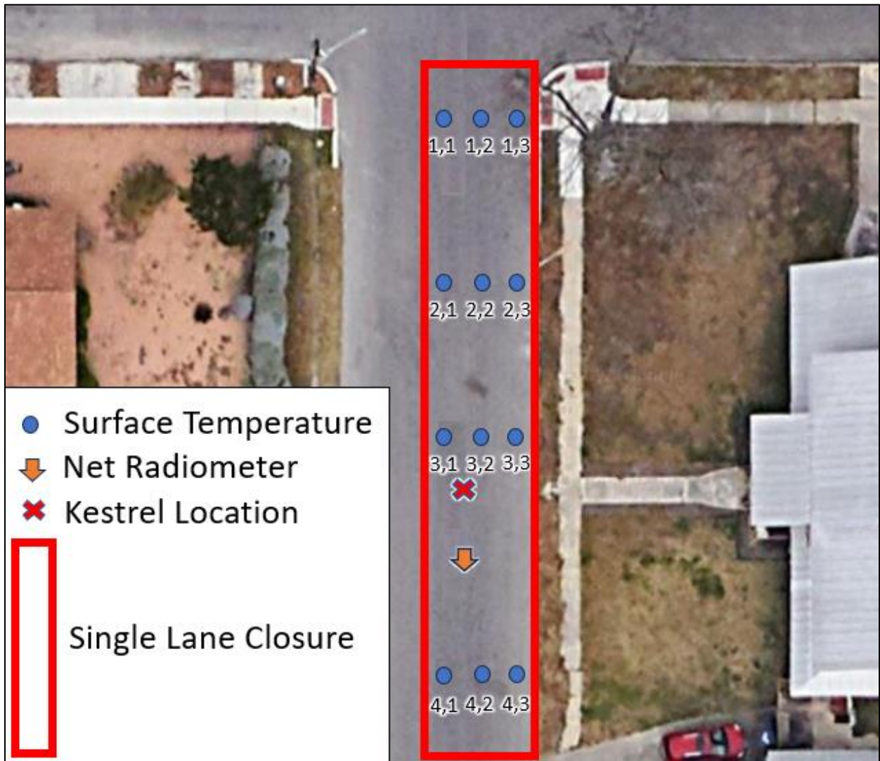
Figure B3. Fieldwork data collection schematic for the Grant Ave. cool pavement site showing the surface temperature grid and Kestrel location during Phase I and the net radiometer location during Phase II (Imagery Source: Google Maps).
