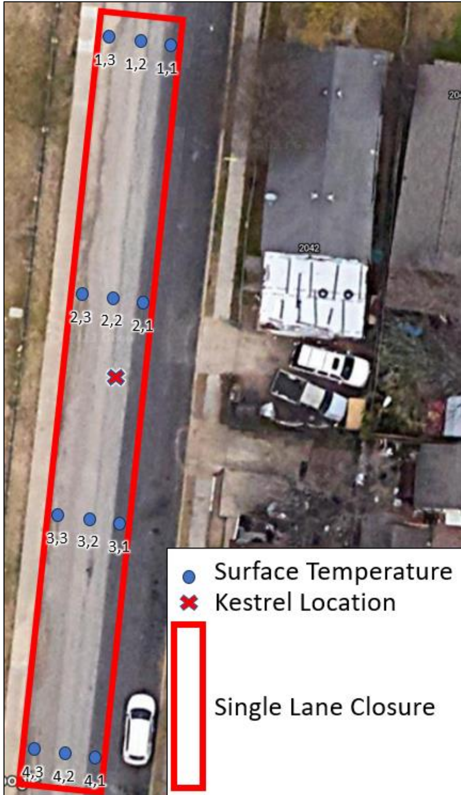
Figure B12. Fieldwork data collection schematic for the SW 21 st St. control site showing the surface temperature grid and Kestrel location during Phase I (Imagery Source: Google Maps).
