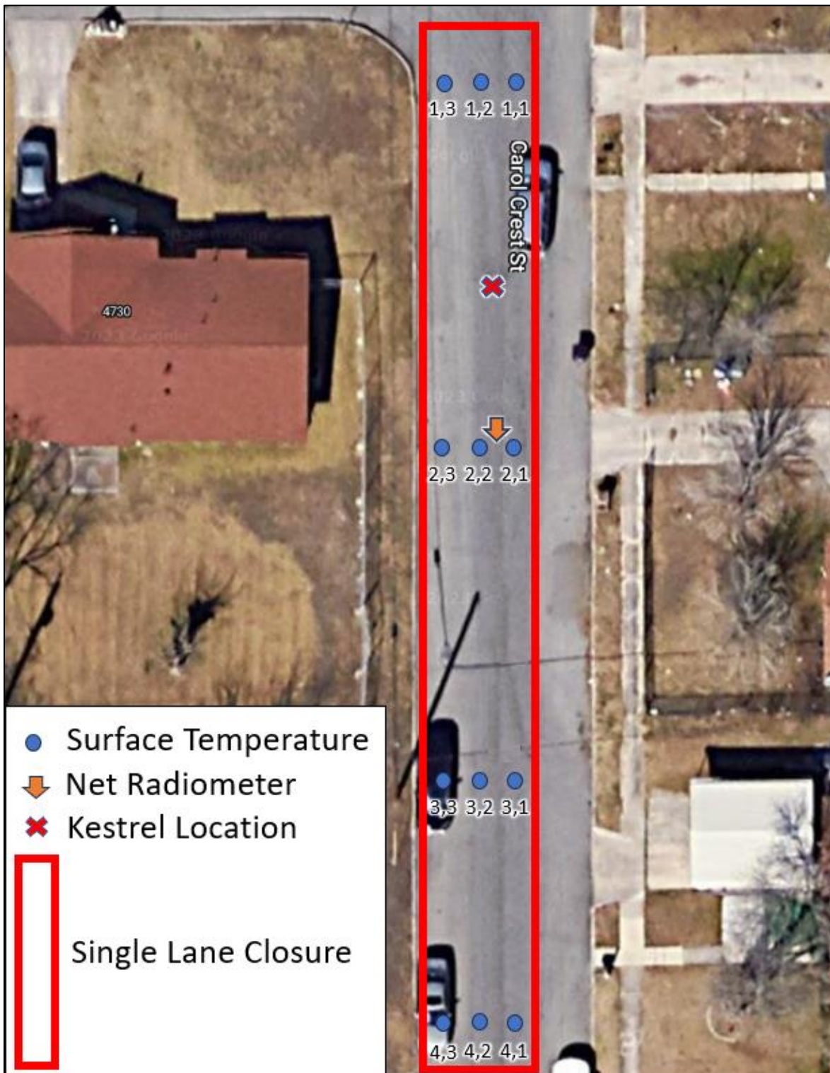
Figure B1. Fieldwork data collection schematic for the Carol Crest cool pavement site showing the surface temperature grid and Kestrel location during Phase I and the net radiometer location during Phase II (Imagery Source: Google Maps).
