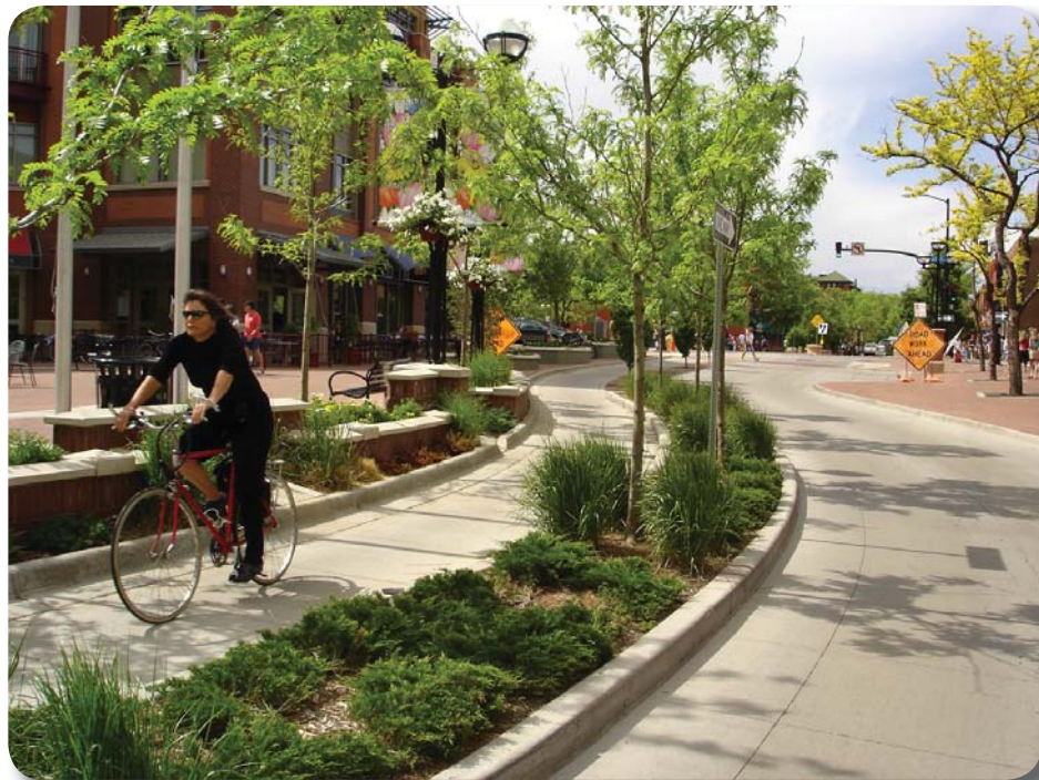
Landscaping between a cycle track and vehicular travel lane Image Source: Toole Design Group
