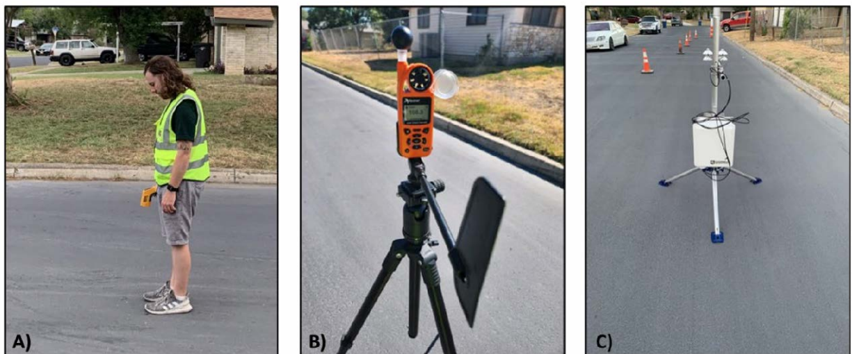
Figure 3. The a) FLUKE 572-2 infrared thermometer, b) Kestrel 5400 Heat Stress Tracker, and c) Hukseflux NR01 4-component net radiometer deployed in the field.
