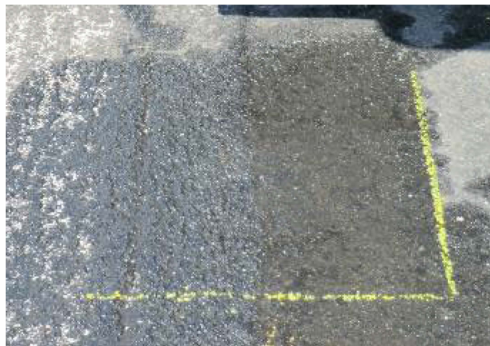
Figure 7. Example of marking from the CT Meter to align DF Tester in the same location.
