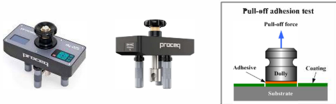
Figure 4. Pull-off tester and diagram of the adhesion test procedure.
