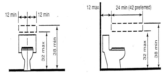
Location of Grab Bar Reinforcements for Adaptable bathrooms NOTE: The areas outlined in dashed lines represent locations for future installation of grab bars for typical fixture configurations.
