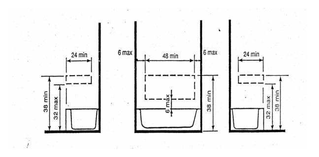
Location of Grab Bar Reinforcements for Adaptable Showers NOTE: The areas outlined in dashed lines represent locations for future installation of grab bars for typical fixture configurations
