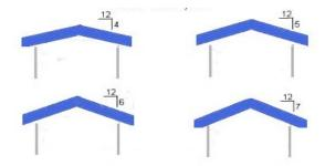
The illustration shows variations of a moderate roof pitch. A moderate pitch has a shallow slope.
