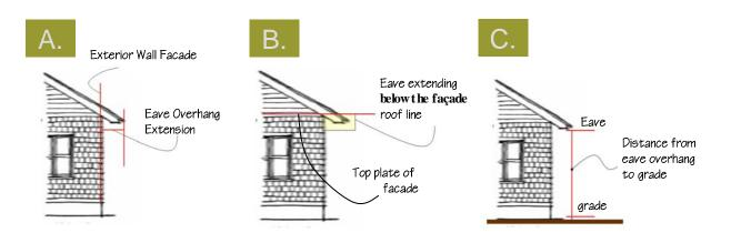
The illustrations above provide examples for determining and measuring the eave overhang. The design and style of roof eave dimensions helps compliment the desired roof orientation, scale and proportion of the roof pitch.
