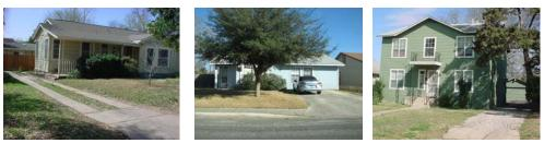
An appropriate driveway configuration locates the automobile to the side of the primary dwelling structure. Terminating a front driveway or placing a parking pad at any non-parking structure is prohibited.
