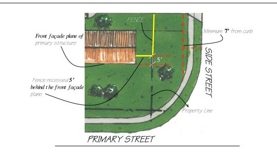
Side yard fencing shall be recessed at least seven feet from the side street curb. In most cases, the property line will extend greater than the minimum seven foot distance requirement.
