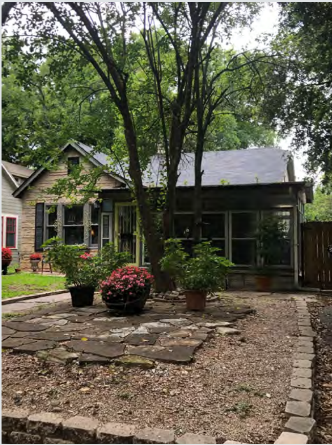
Figure 4.7.3. Example of a yard with 50 percent of the historic lawn area replaced with hardscaping, using a combination of impermeable materials (flagstone) and permeable materials (gravel). Replacement of the flagstone with either landscaping or a permeable material like gravel or mulch is recommended but not required. Source: Photo by HHM, 2021.
